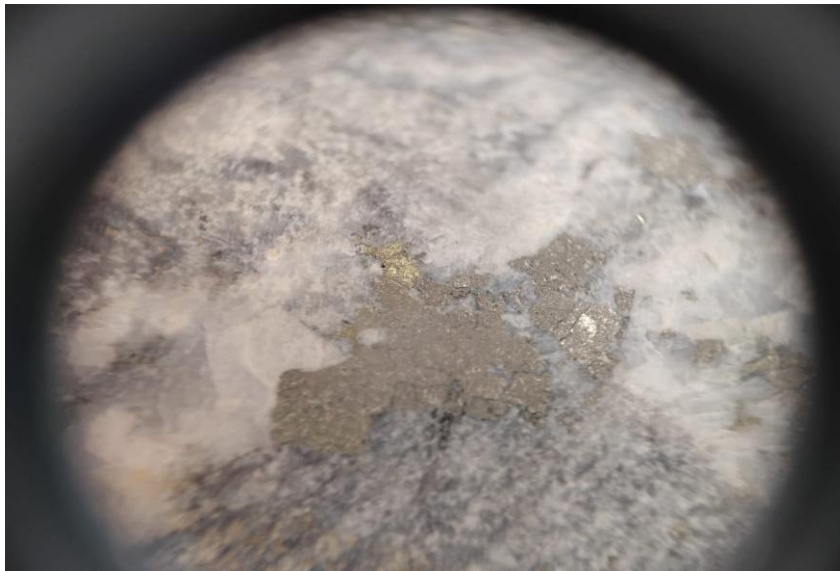
Image 2: Chalcopyrite grain (yellow) in contact with pyrite (brassy). Chalcopyrite serves as a strong indicator mineral in the deposit.
